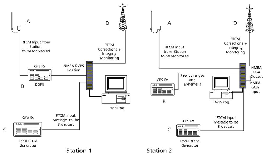
Station 1: DGPS position computed by GPS receiver
