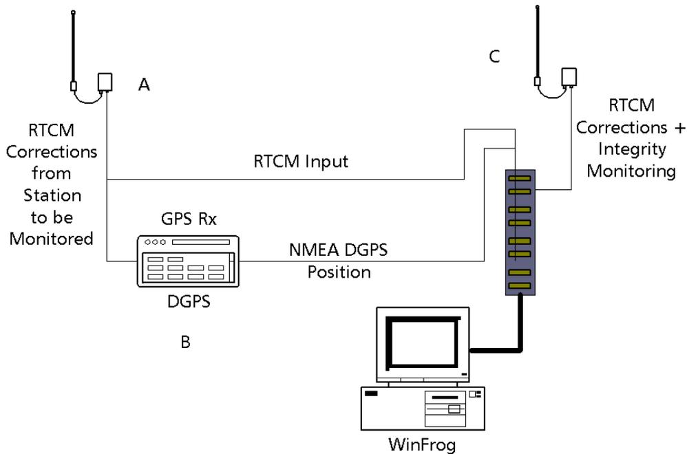
As shown above, a single base station RSIM system requires three main components:
